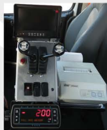
*Patent Pending ergonomic control console that includes: rear camera monitor, hoist controls, work light switch, PTO switch, and optional on-board scale digital read-out and printer
