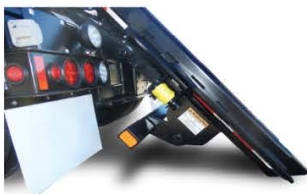
Mechanical forward folding ICC Bumper (Can be pinned up for trailering)
